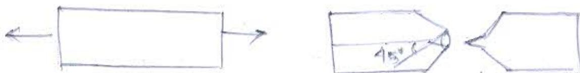
Since ductile material weak in shear, therefore failure is due to shear. Failure plane is at  $45^\circ$  from longitudinal axis. Such type of failure is known as shear-cone failure.
