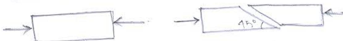
Since the brittle material is strong in compression therefore it will fail in shear. The angle of failure plane is at  $45^\circ$  from longitudinal axis.
